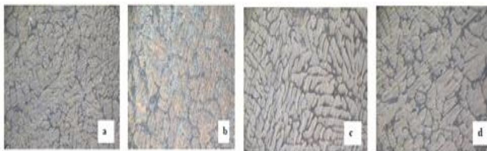
Fig. 10. Micrographs showing red mud distribution in the composites of different Volume fractions (a) 10% (b)15% (c) 20% and (d) 30% at (200 X)
